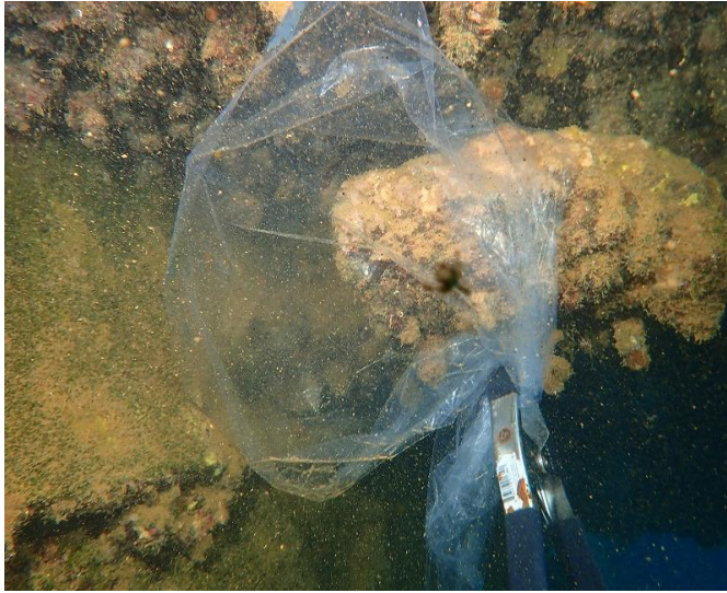
Image 2: Plastic covering of vent to measure amount oil, approximately 200cc in 10 minutes.
