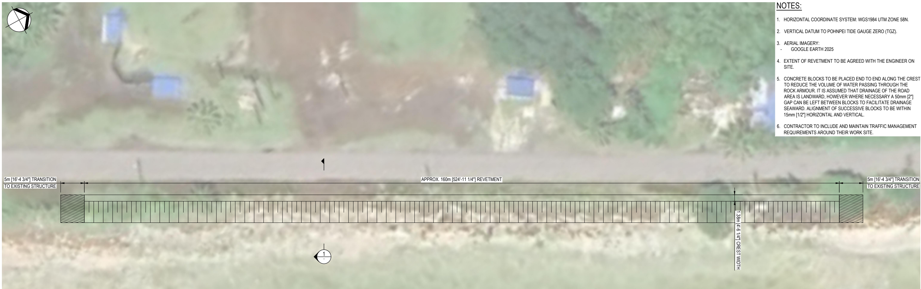
PAAL NORTH REVETMENT GENERAL ARRANGEMENT PLAN SCALE 1:250
