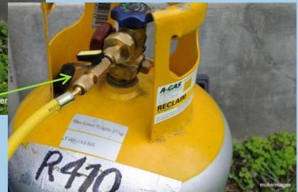
Isolation couplers are used to eliminate emissions
