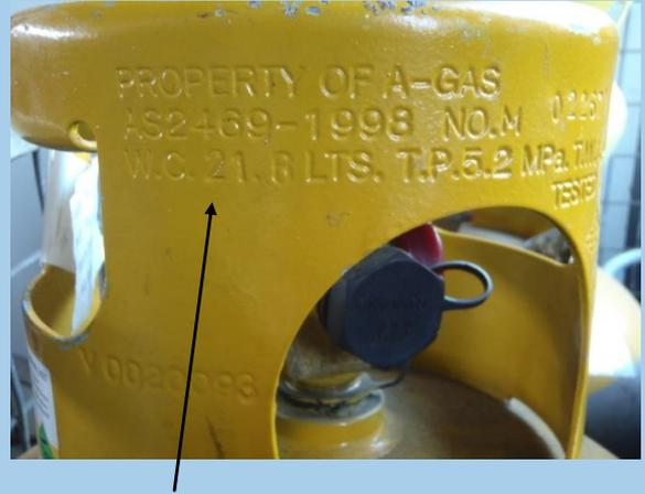
**Water Content** (amount of water in weight that the cylinder can hold)
