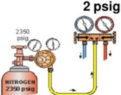
The diagram shows a nitrogen cylinder on the left with a pressure gauge reading 2350 psig. A yellow hose connects the cylinder to a manifold on the right. The manifold has two gauges and is labeled 2 psig. A yellow arrow points from the manifold back towards the cylinder, indicating the direction of flow.
