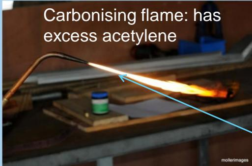
Carbonising flame: has excess acetylene
