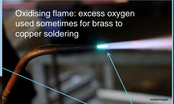
Oxidising flame: excess oxygen used sometimes for brass to copper soldering
