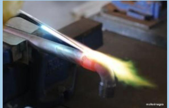
When soldering always purge with nitrogen : this reduces the build up of oxidising agents inside the tubing.....
