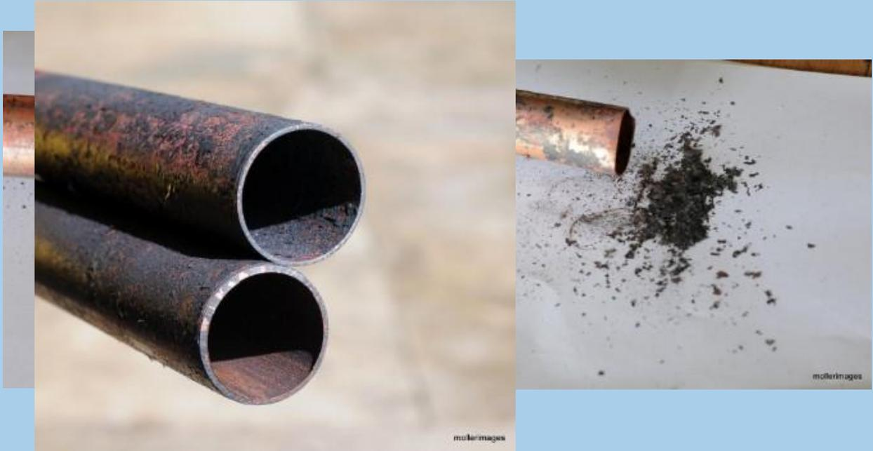
This is the result annealing two identical tubes, one purging with nitrogen one without
