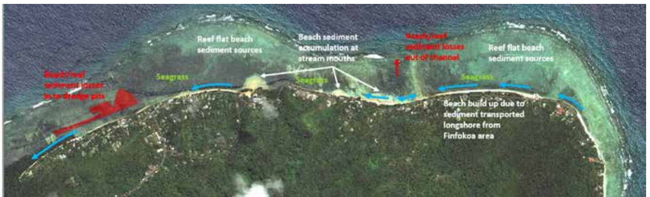
Figure B 3: Key sediment sources, longshore transport processes, and sediment losses along the Tafunsak shoreline.
