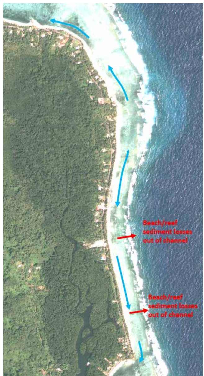
Figure B 10: Key sediment sources, longshore transport processes, and sediment losses along the Pukusruk shoreline.
