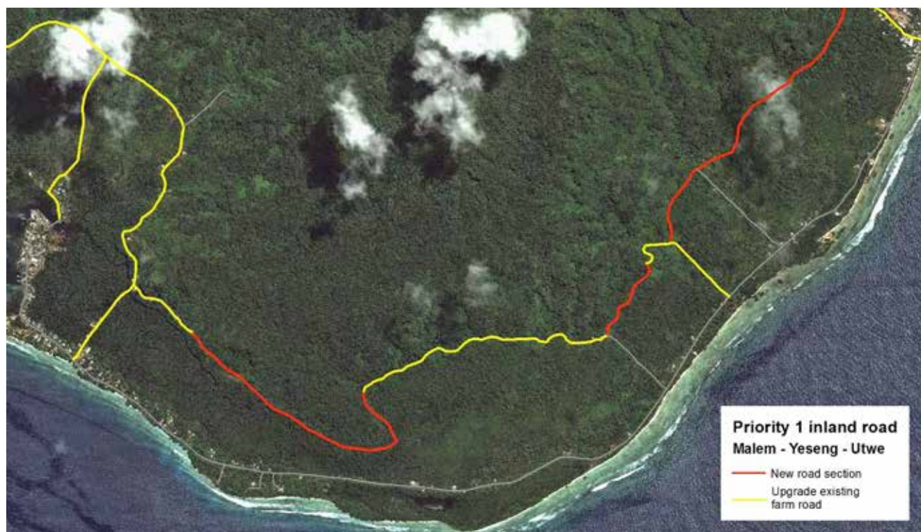
Figure 15: Indicative inland road between Utwe and Malem showing the requirements of new and upgraded sections of road.
