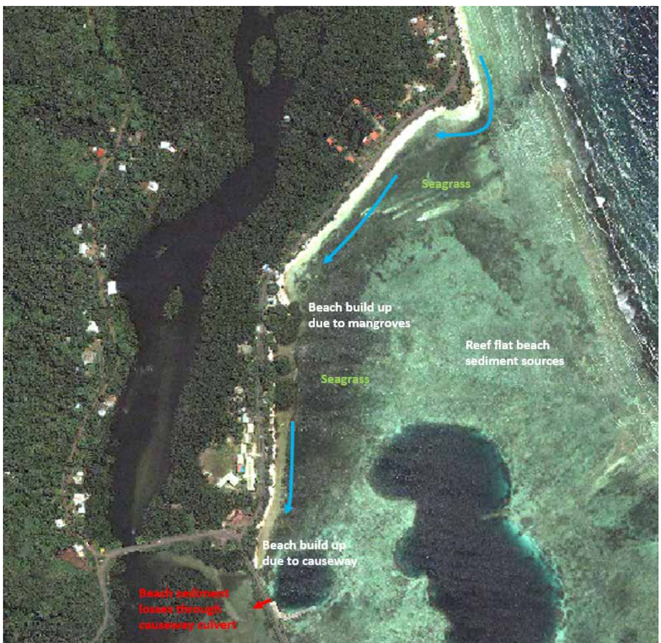
Figure B 5: Key sediment sources, longshore transport processes, and sediment losses along the Putukte to Finpukal shoreline.
