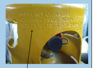
Water Content (amount of water in weight that the cylinder can hold) W.C. x .8 = Safe Refrigerant capacity 21.8x.8 = 17.5KGs of recovered refrigerant can be safely added to the cylinder
