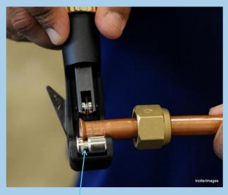
Notice groove in cutting wheel to fit flare
